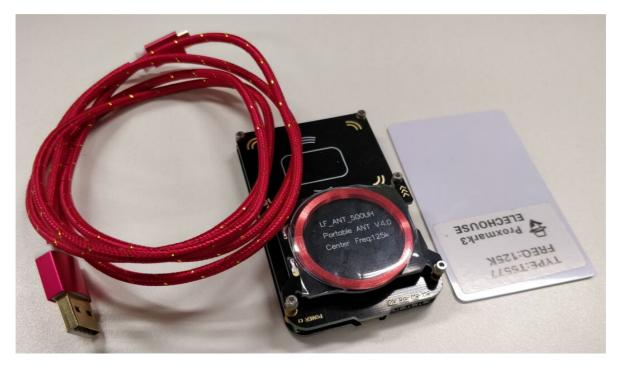
According to its readme page, "The proxmark3 is a powerful general-purpose RFID tool, the size of a deck of cards, designed to snoop, listen and emulate everything from Low Frequency (125kHz) to High Frequency (13.56MHz) tags." The source code of Proxmark 3 can be found at <u>https://github.com/Proxmark/</u>proxmark3, Iceman fork(<u>https://github.com/iceman1001/proxmark3</u>) contains more experimental features but is less stable. We use either of them in different situations.
